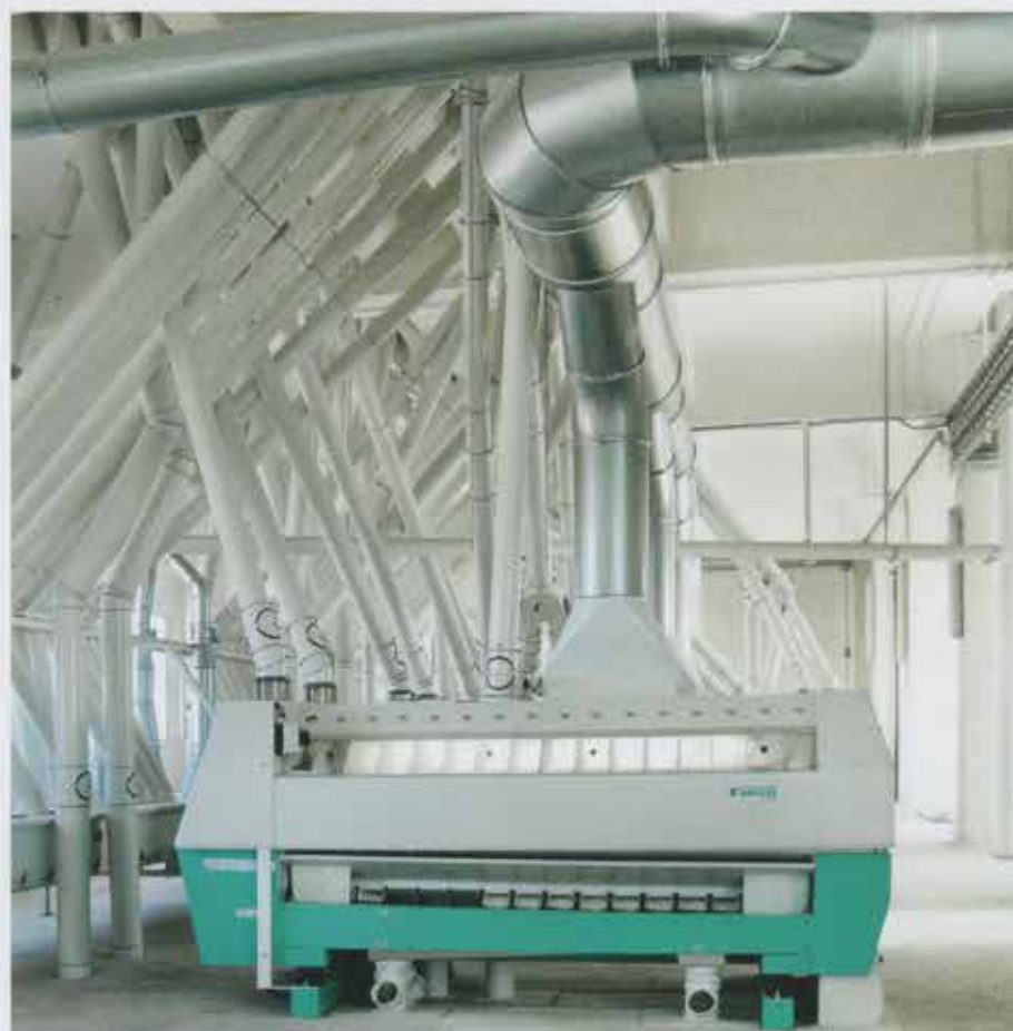
The new South Amman Mills plant operates four purifiers of type MQRF.
